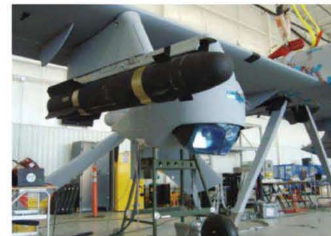
The Triclops flight test will use Raytheon's AN/AAS-53 Common Sensor Payload as the underwing sensors.
